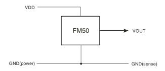
**Figure 4. Recommended Electrical Connections**
