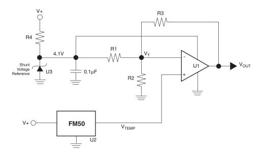
Figure 6. Thermostat/Fan Controller
