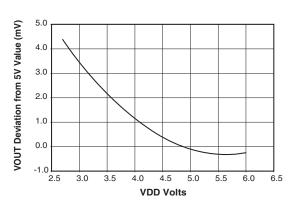
Figure 3. Typical Sensitivity to Supply Voltage
