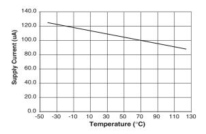
Figure 2. Typical IDD versus Temperature
