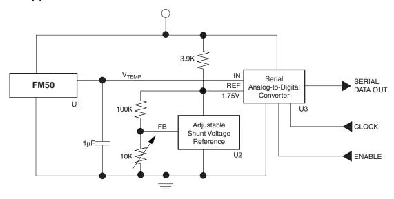
Figure 4. Serial Output Temperature to Digital Converter (Full Scale = +125°C)
