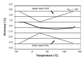
Figure 1. Accuracy vs. Temperature
