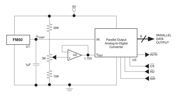
Figure 5. Parallel Output Temperature to Digital Converter (Full Scale = +125°C)
